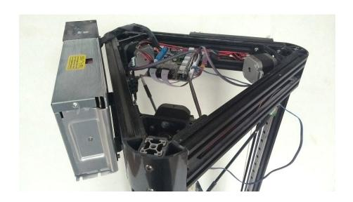
Follow the build instructions until you get to the Filament holder and Extruder motor. The filament holder is not attached and the Extruder motor, minus the mount is used to make the Clay Printhead - see next section. The Anycubic Plastic printhead is removed from the printhead mount plate and your Clay Printhead will later get attached to this plate. The plastic printhead is not used and is pre-assembled on the printhead plate that is attached to the diagonal rods.
