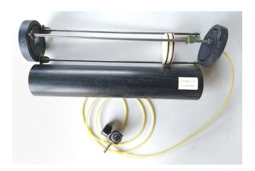
An improvement that I would suggest should be made on the black container design is to have four long rods rather than three rods that hold the two end caps together along the length. The container is put under 4 – 6 Bar of pressure and with only three bracing/connecting rods the end plates bend ever so slightly and the air pressure leaks out. With four bracing rods placed around the circumference of the endplates this could be bolted up more evenly.
