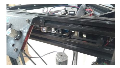
The Power supply I mounted horizontally and up away from any water. The wires just reach the mainboard.
