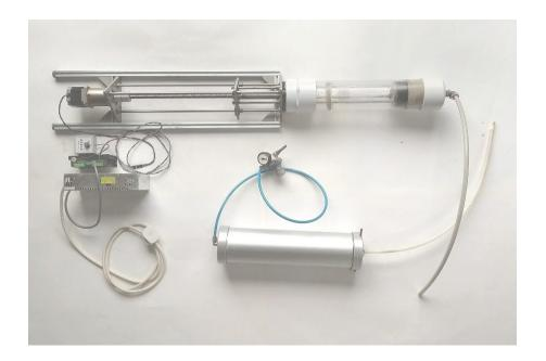
I do also have a mechanical ram per kind favour of <u>ClayBot</u> so I have run my Anycubic with both a ram clay delivery and the compressed air delivery. Both work well but I prefer the simplicity of the air system. I would use the same consistency of clay in either system. In the photograph above the air pressure container (lower middle) holds more clay than the ram above and is easier to clean and maintain.
