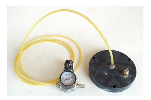
This is the endplate where the air comes in. A push connector holds the air line coming from the pressure regulator. I print at between 4-6 bar of pressure. The brass fitment to the right on the end cap is a safety pressure valve that that I am told will release pressure above 8 bar of pressure. A very important safety feature.
