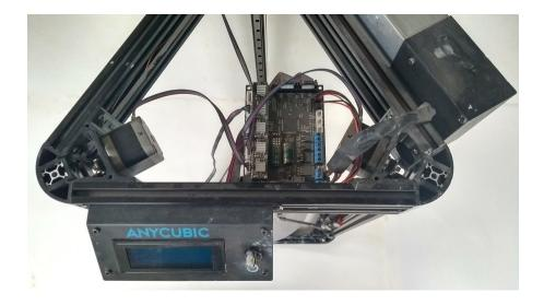
I did move the mainboard along so I could access the usb input next to the display screen. The display screen is mounted left of centre.
